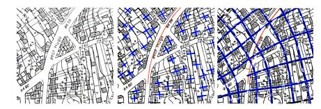
Example South East of Paris (Seine Amont Orly Airport) : grid is parallel or perpendicular to the slopes [water flows and drainage]
